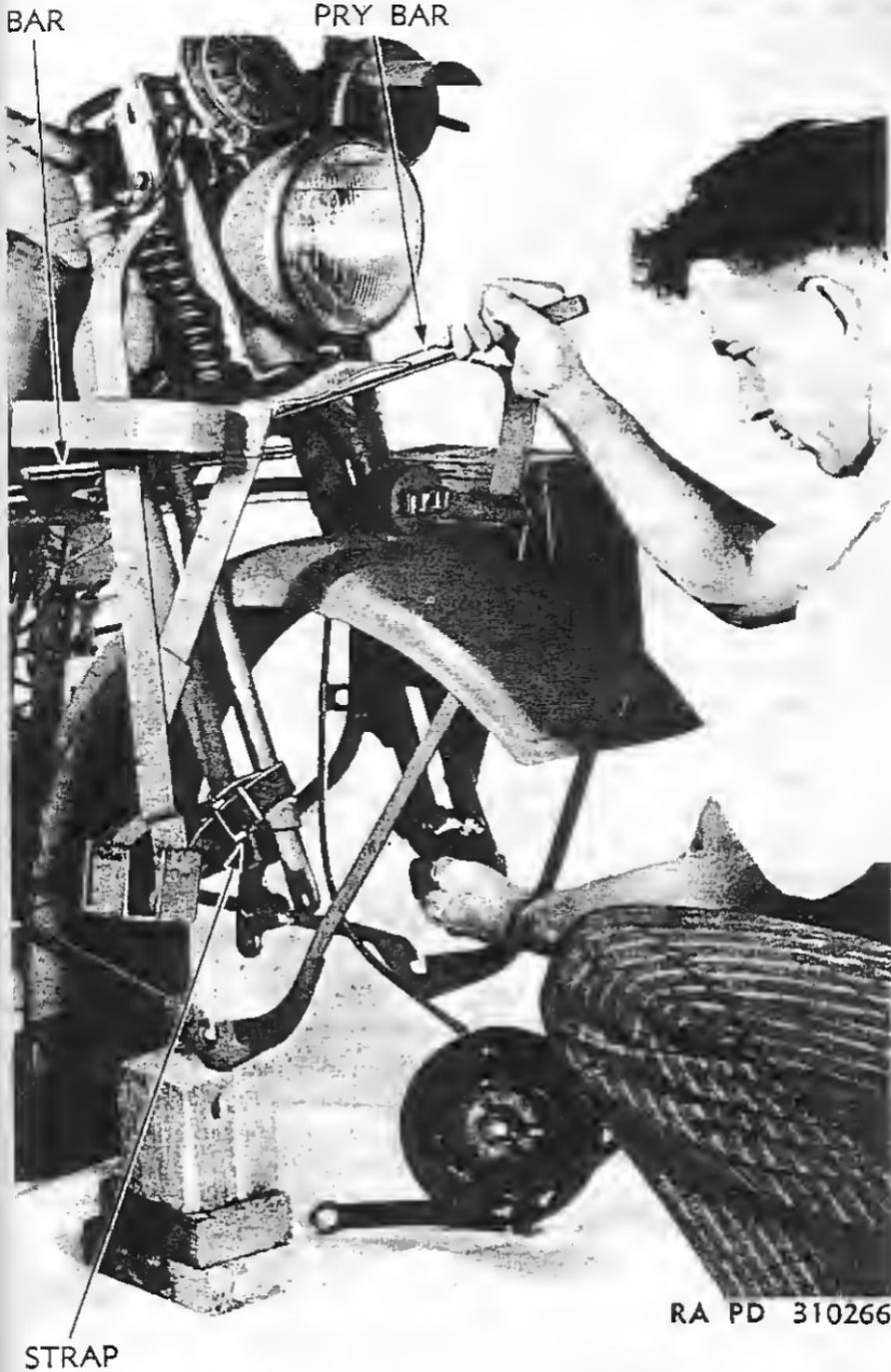
**Figure 64—Compressing Cushion Springs for Spring Fork Assembly**
