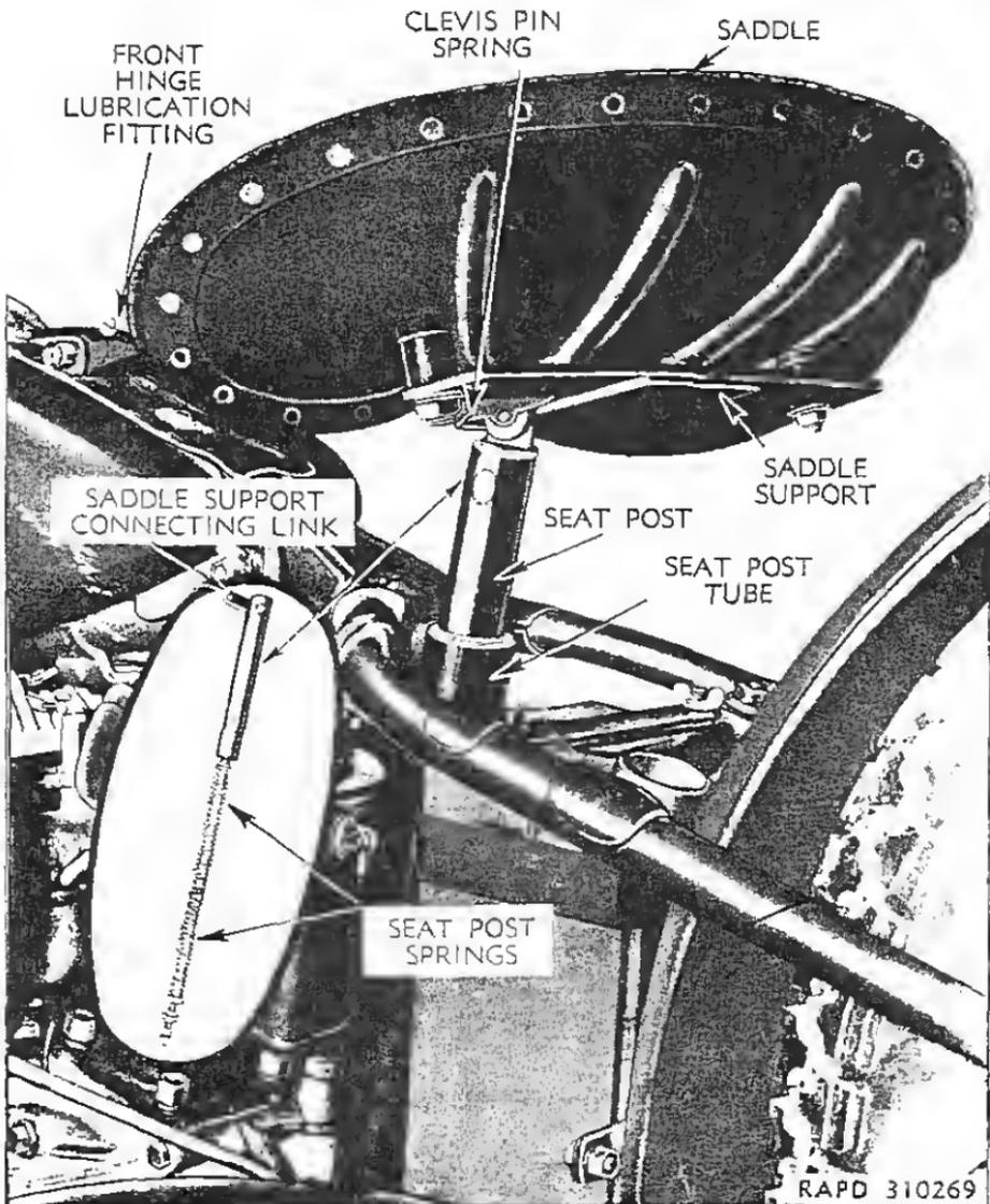
**Figure 71—Saddle and Suspension**
