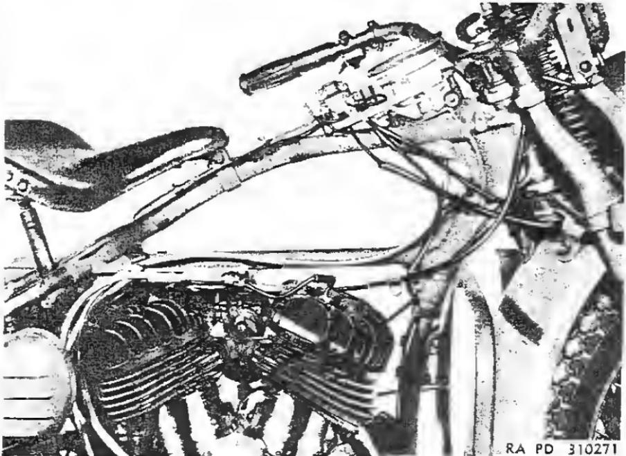
*Figure 79—Wiring Cables, Right Side*
