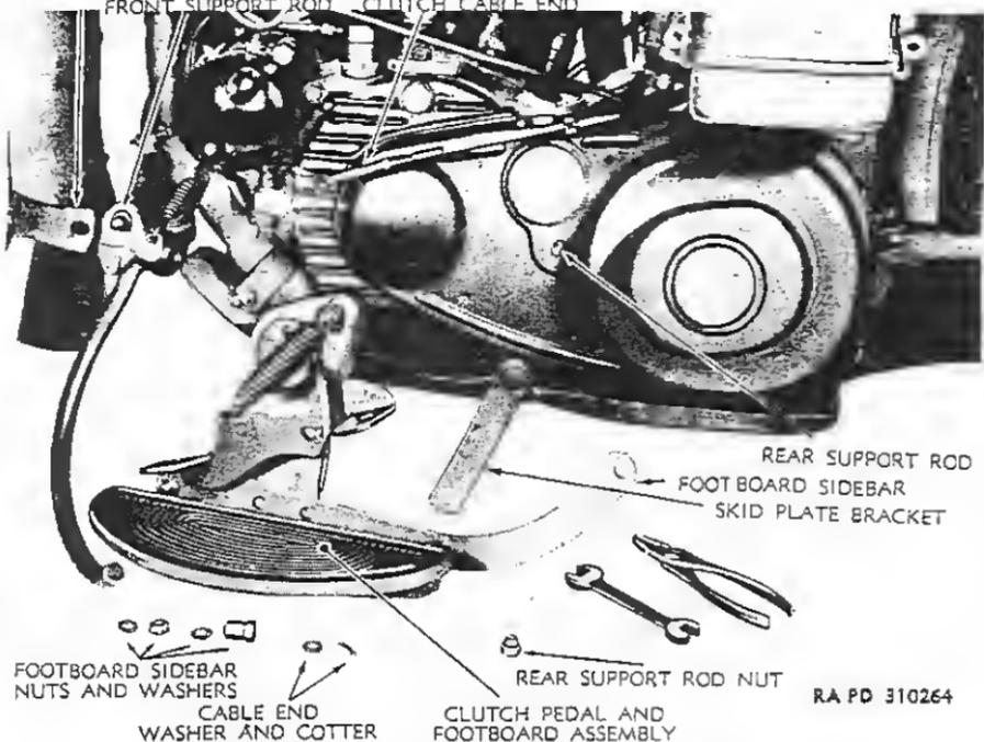
**Figure 68—Left Footboard Assembly Removed**
