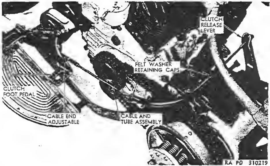
*Figure 22—Clutch Control Linkage*
