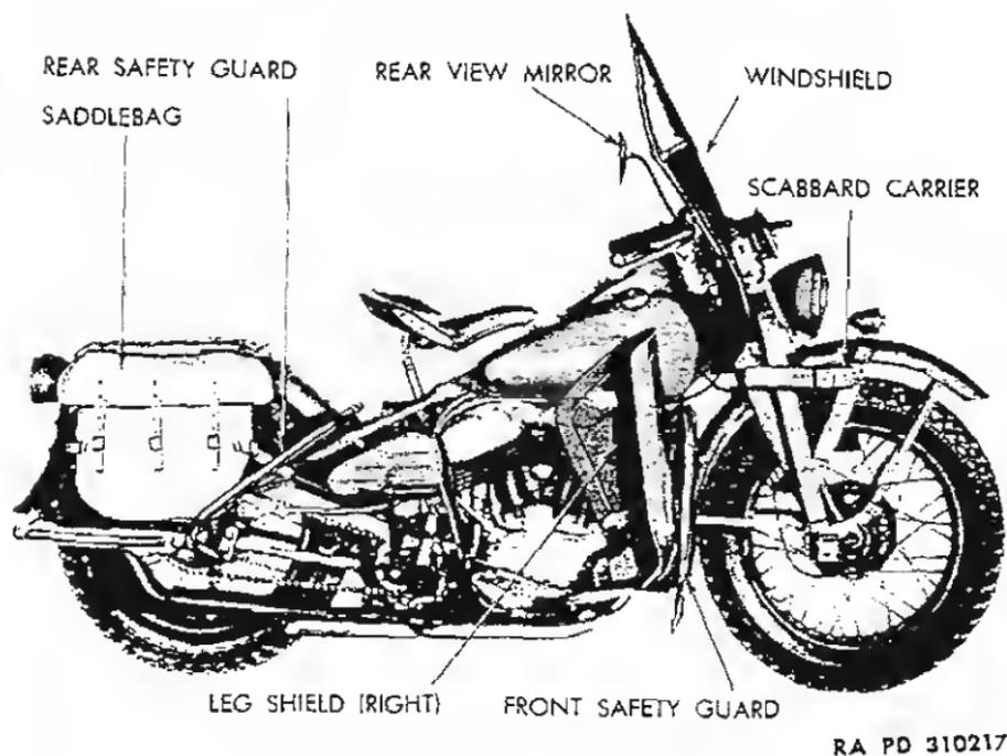
*Figure 13—Vehicle Equipment, Right Side*
