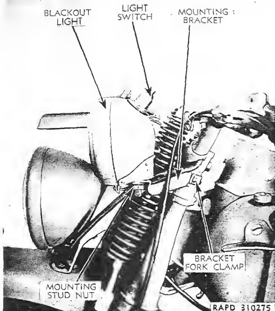
**Figure 75—Blackout Headlight Installation**
