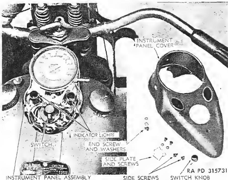
**Figure 80—Panel Cover Removed**
