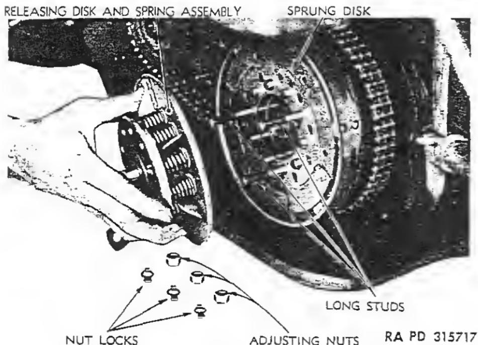
Figure 29—Outer Assembly Removed, Exposing Clutch Disks
