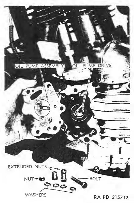
Figure 17-Oil Pump Removed 76
