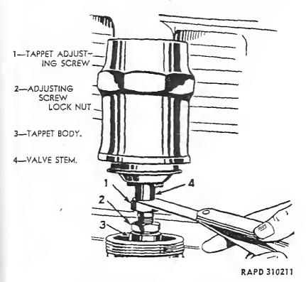
Figure 16-Valve Tappet Adjustment
