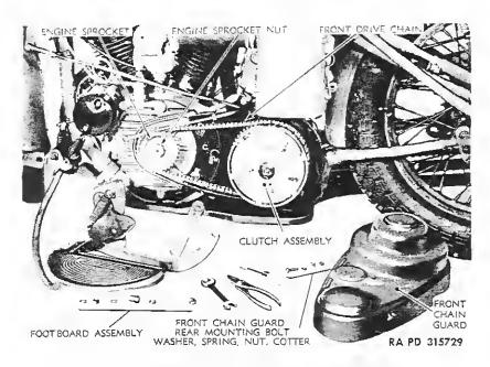
Figure 69—Outer Front Chain Guord Removed
