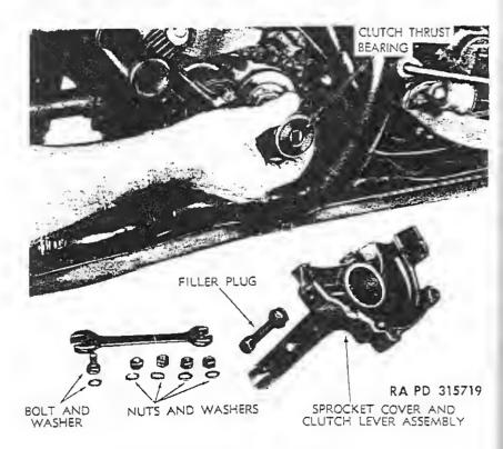
Figure 31—Removing Clutch Releasing Bearing Assembly
