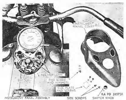
Figure 80-Panel Cover Removed
