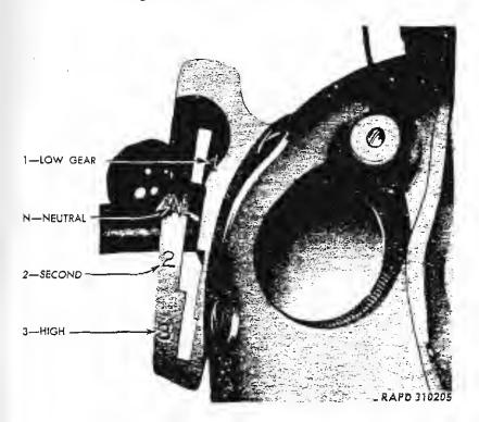
Figure 8—Gear Shifter Lever Positions
