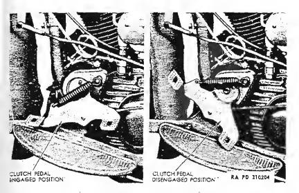
Figure 7-Clutch Pedal Positions
