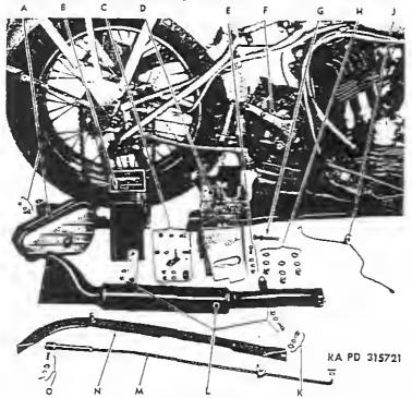
A-TOOL BOX AND BRACKET ASSEMBLY AND MOUNTING BOLT, WASHER AND NUT
