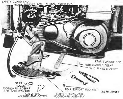
Figure 68-Left Footboard Assembly Removed
