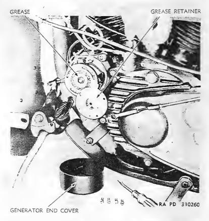
Figure 57—Generator End Cover and Grease Retainer Removed
