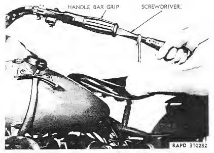
Figure 66-Removing Handle Bar Grip Sleeve Retaining Nut
