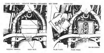
Figure 74—Battery Bax Open and Filler Plugs Removed for Service
