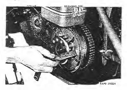
Figure 27—Measuring Distance Between Spring Callar and Disk
