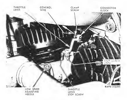
Figure 44-Throttle A Fully Open Position
