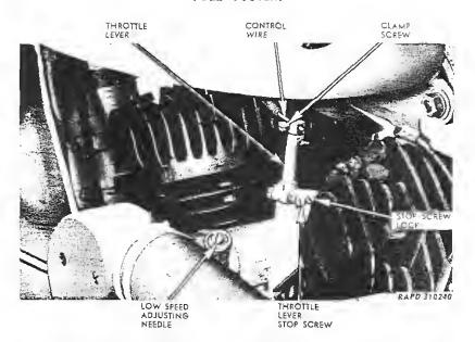
Figure 43-Throttle In Fully Closed Position
