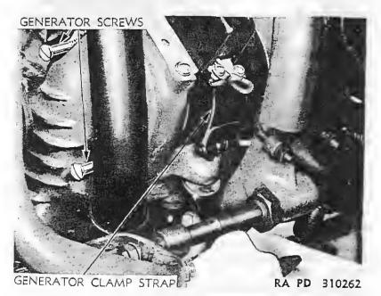
Figure 59-Removing Generator Strop Nut 146
