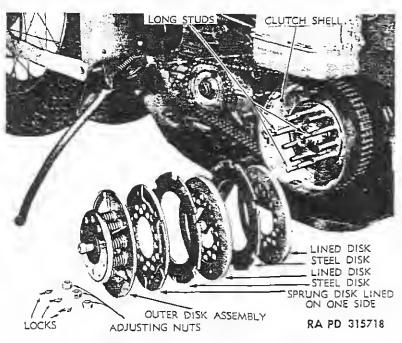
Figure 30—Clutch Disks, Removed
