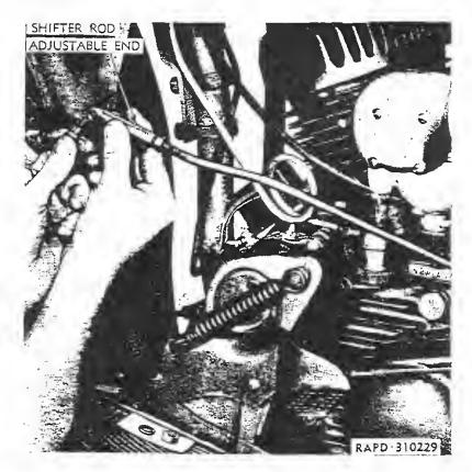
Figure 32-Adjusting Gear Shifter Rod
