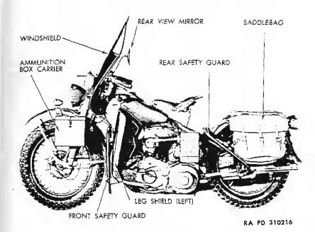
Figure 12-Vehicle Equipment, Left Side
