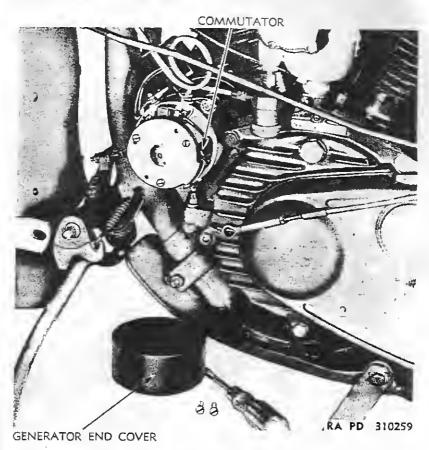
Figure 56-Generator Caver Removed for Commutatar Cleaning
