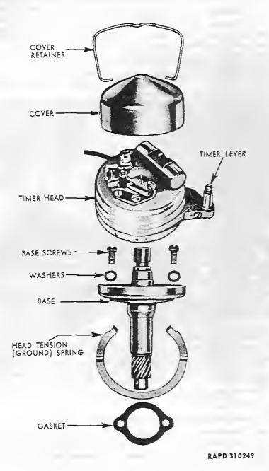
Figure 50—Circuit Breaker (Timer), Disassembled
