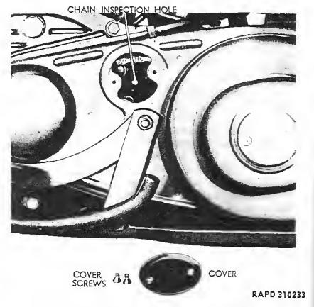
Figure 36-Front Chain Inspection Hole Cover Removed
