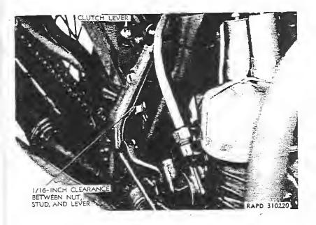
Figure 23-Clutch Lever and Stud Nut Clearance
