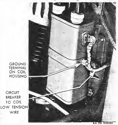
Figure 53—Shielded Coil to Timer Wire Correctly
