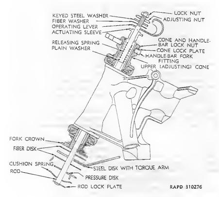
Figure 65-Steering Damper Assembly
