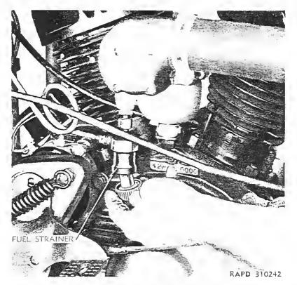
Figure 45-Removing Fuel Strainer
