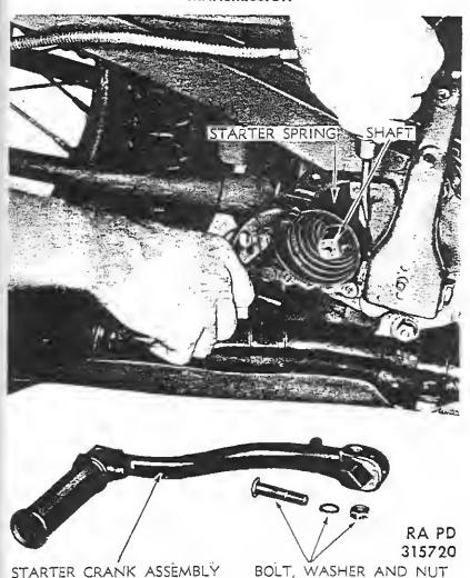
Figure 33-Removing Starter Crank Spring
