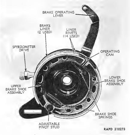
Figure 61-Rear Brake Assembly
