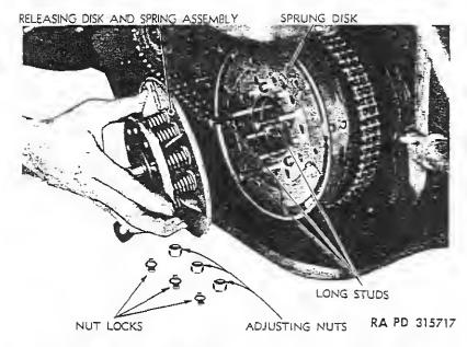
Figure 29-Outer Assembly Removed, Exposing Clutch Disks
