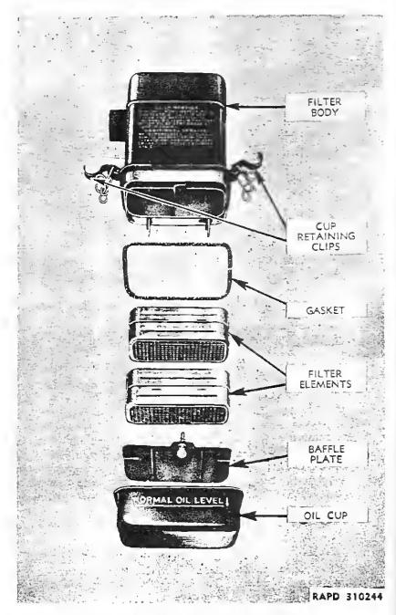
Figure 47—Air Cleaner, Disassembled
