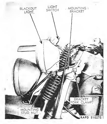
Figure 75-Blockout Headlight Installation
