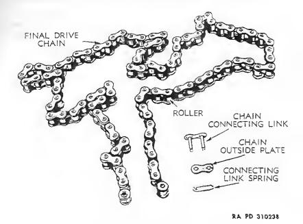
Figure 41—Rear Drive Chain and Connecting Link
