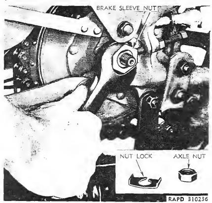
Figure 39-Brake Sleeve Nut
