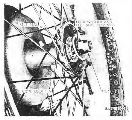
Figure 82-Front Hub Prepared for Cone Adjustment
