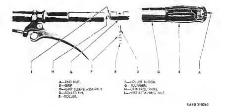
Figure 67—Handle Bor Grip and Wire Control, Disassembled
