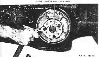
Figure 26—Adjusting Clutch Spring Tension
