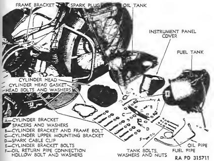
Figure 15—Disassembly for Head Gasket Replacement
