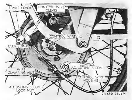
Figure 62—Front Brake Control and Adjusting Members
