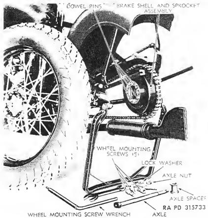
Figure 83-Disassembly for Rear Wheel Removal
