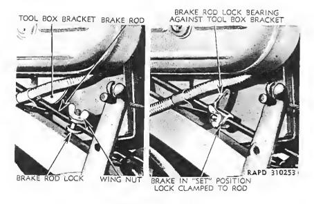
Figure 84—Brake Rod Lock
