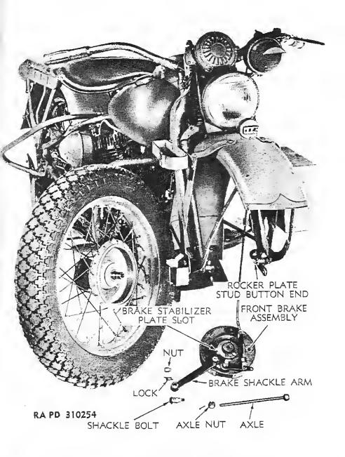
Figure 81—Disassembly for Front Wheel Removal
