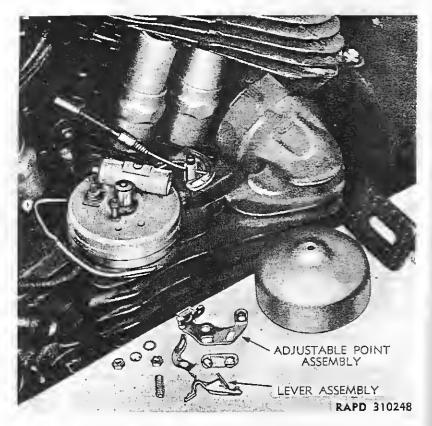
Figure 49-Circuit Breaker Points Removed
