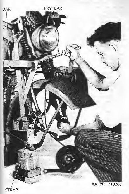
Figure 64—Compressing Cushion Springs for Spring Fork Assembly
