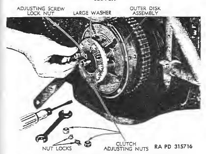
Figure 28-Removing Spring and Outer Disk Assembly
